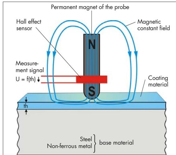
Schematic diagram of the magnetic test method. The indentation depth of the magnetic field depends on the permeability of the base material.
