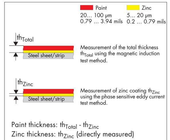
Determining the single coating thicknesses at the duplex measurement using the phase sensitive eddy current and the magnetic induction test methods
