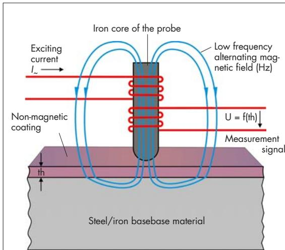
Schematic diagram of the magnetic induction test method. The indentation depth depends on the permeability of the base material.
