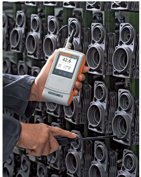
Measuring with the internal probe FAI3.3-150
