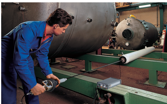
Testing of the interior coating of a pipe with a rotating electrode on a rod system and the POROSCOPE®
